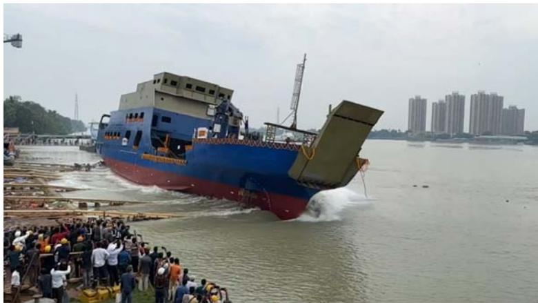
FIGURE 2 SIDE LAUNCH OF MONO HULLED (SINGLE HULL) PASSENGER CUM CARGO FERRY, MV MA LISHA, AT TITAGARH RAIL SYSTEMS LIMITED ON THE BANKS OF HOOGHLY RIVER. THE HEEL (TILT) OF THE SHIP POST LAUNCH IS EXPECTED AND A RIGHTING MOMENT CREATED AS A RESULT OF BUOYANCY FORCE ACTING UPWARDS BRINGS THE SHIP BACK TO ITS UPRIGHT POSITION IN ORDER TO ATTAIN EQUILIBRIUM.
