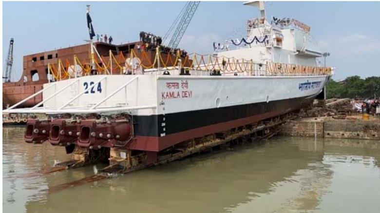
FIGURE 1 END LAUNCH OF FAST PATROL VESSEL, ICGS KAMALA DEVI, AT TITAGARH RAIL SYSTEMS LIMITED (KOLKATA) ON THE BANKS OF HOOGHLY RIVER. THE SLIPWAYS CAN BE SEEN BELOW THE SHIP.
