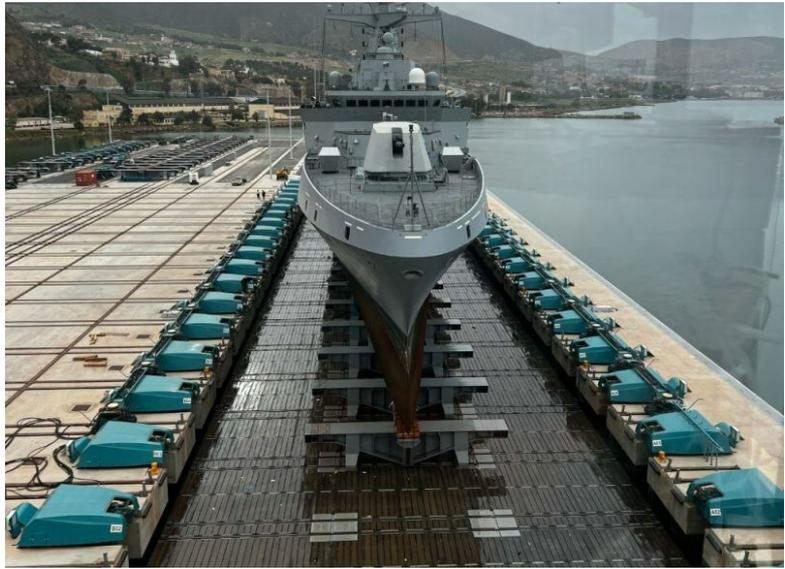
FIGURE 9 EXAMPLE OF A SYNCROLIFT
