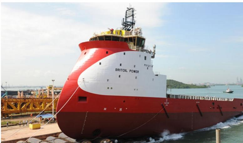
FIGURE 7 LAUNCH OF PLATFORM SUPPLY VESSEL (PSV), BRITTOIL POWER, USING AIRBAGS. NOTICE THE INVERTED BOW HULL SHAPE AT THE FRONT. THIS IS CALLED THE 'ULSTEIN X-BOW' DESIGNED AND DEVELOPED BY THE ULSTEIN GROUP. THIS SHAPE AIDS IN REDUCING FUEL CONSUMPTION DUE TO LOWER HYDRODYNAMIC DRAG.
