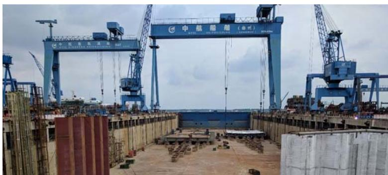
FIGURE 4 DRY DOCK AT AVIC DINGHENG SHIPBUILDING CO. LTD., YANGZHOU, CHINA. TWO SHIPS UNDER THE ASSEMBLY PHASE CAN BE SEEN IN THE PICTURE WITH A DOCK GATE AT THE END.
