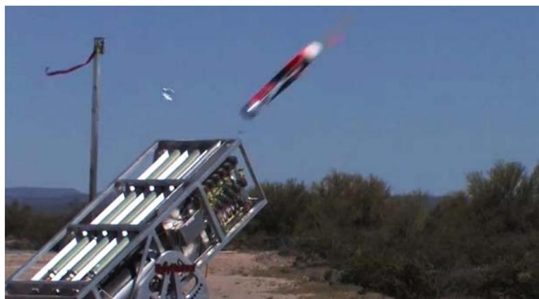
Fig 2 : US Navy LOCUST Tubular Autonomous Swarming UAV
