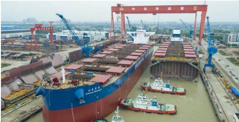
FIGURE 5 DRY DOCK AT COSCO SHIPPING HEAVY INDUSTRIES CO. LTD., YANGZHOU, CHINA. FLOODED DRY DOCK WITH THE SHIP BEING FLOATED OUT OF THE DOCK WITH THE AID OF PUSH & PULL TUG BOATS.
