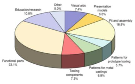
Fig.2: Application areas that AM is currently being used for, courtesy of Wohlers Associates
